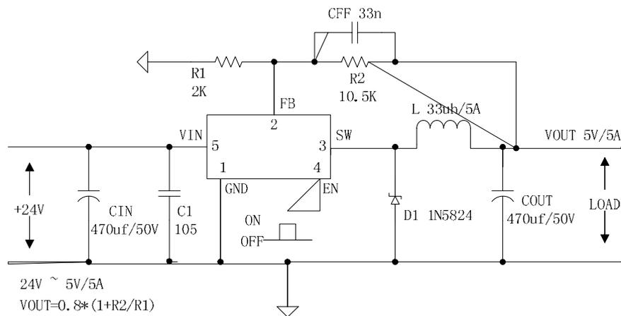
Figure7. GS2678 System Parameters Test Circuit (24V ~ 5V/5A)
