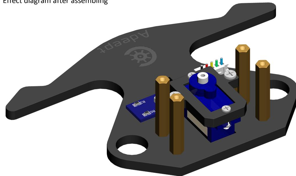
7. Connect the rocker arm of a servo with A07.
