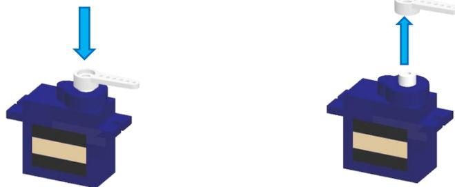
Rotate the rocker arm between 0 and 180 degrees.
