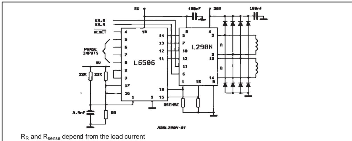
R<sub>R</sub> and R<sub>sense</sub> depend from the load current
