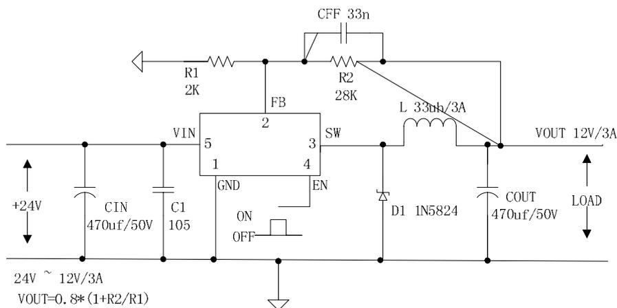
Figure6. GS2678 System Parameters Test Circuit (24V ~ 12V/3A)
